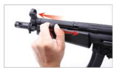
Pull the Charging Handle backward and release it. The gun is ready to fire.
