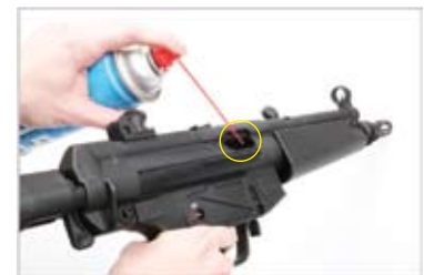
Use airsoft safe silicone to lubricate the hop-up chamber. Use silicone lubricant sparingly.
