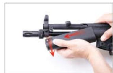
1. Pull the handguard downwards. 2. Slide the handguard forward and remove form the gun.
