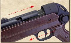
5. Assemble the upper and lower receiver by pushing them in the same direction
