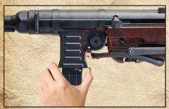
1. Push the magazine release button and remove the magazine
