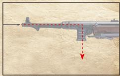
3.Insert the cleaning rod into the barrel to remove the jammed BBs
