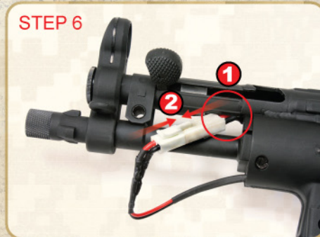
1. Let the battery lead passes through the hole. 2. Connect the battery leads.
