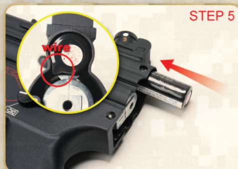
Insert the battery into the upper receiver. (Please note the wire, when you insert the battery)
