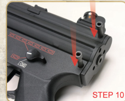
Reinstall the locking pins
