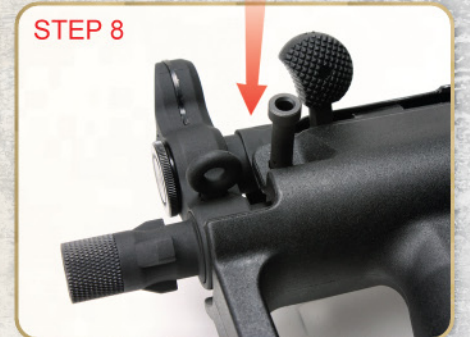
Reinstall the locking pin
