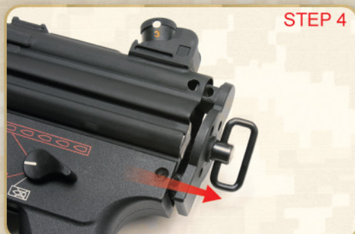
Remove the butt cap.
