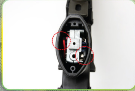
Please check the motor wiring connections.
