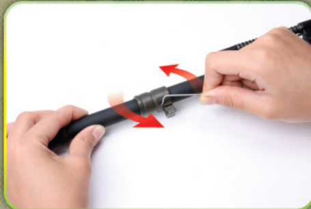
Release the Bayonet mount use allen key(1.5mm).
