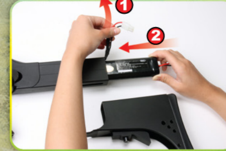
1.Pull the battery lead from stock . 2.Insert the Battery.
