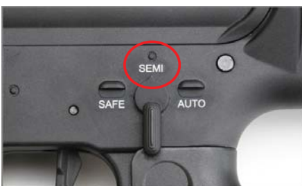
⚠ Turn the Selector to semi (將設定鈕切換到單發模式)
